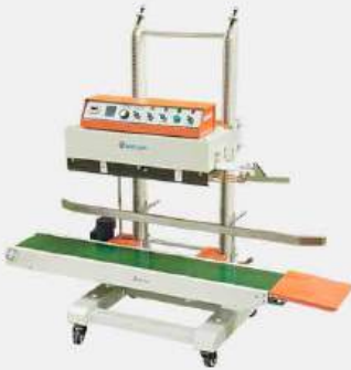
Continuous Band Sealing Machine (MS Body) Load Capacity : 25kg Sealing Width : 10-12mm
